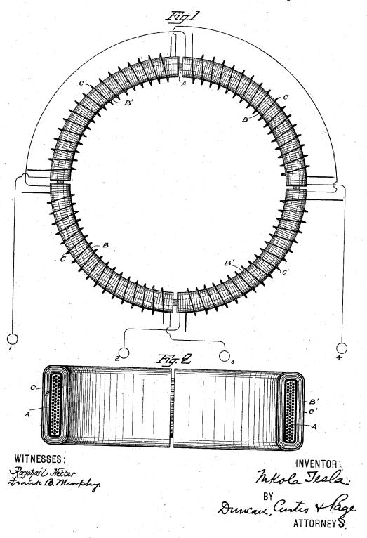
METHOD OF CONVERTING AND DISTRIBUTING ELECTRIC CURRENTS.
